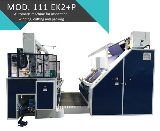
The model Eureka 2 is an automatic machine suitable to inspect, wind, cut and pack rolls of fabric. This machine is the heart of Testa production, being today the best-selling model, thanks to its versatility. In addition to the cycles listed above, the peculiar feature of this machine consists in the possibility of automatically discard the defective fabric, the seams or the sample fabric, along a belt placed underneath the machine itself, without interrupting the other machine cycles.
